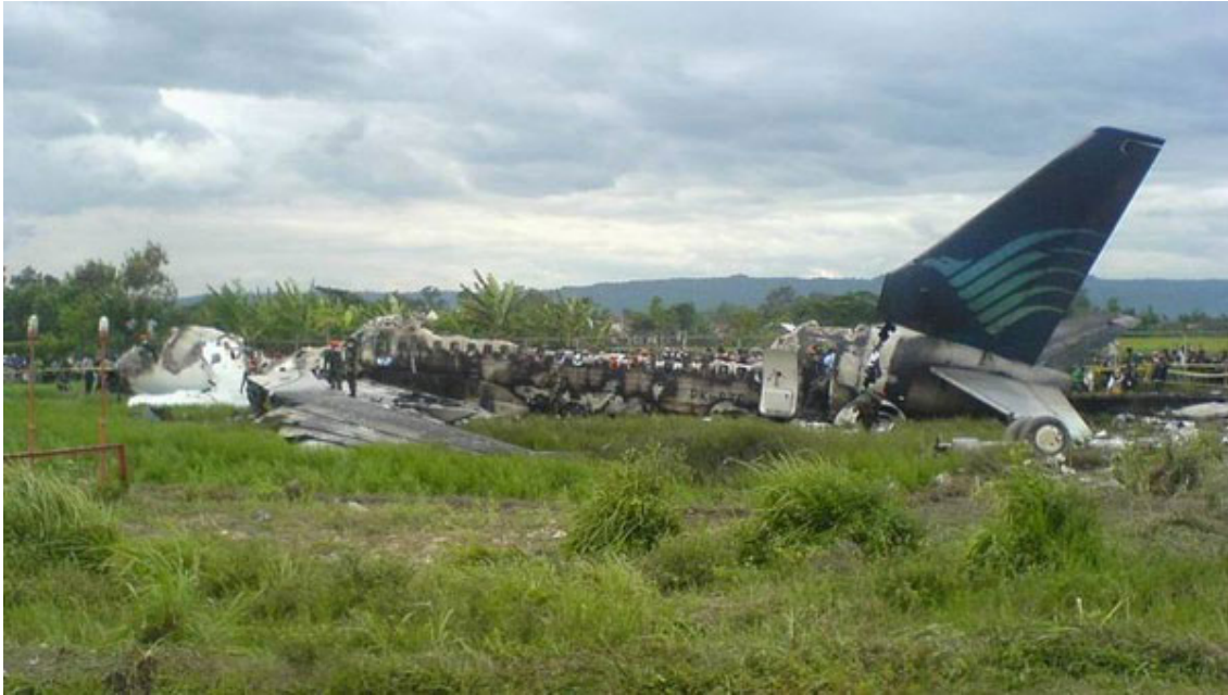
Fire had destroyed most of the fuselage (detik.com)
