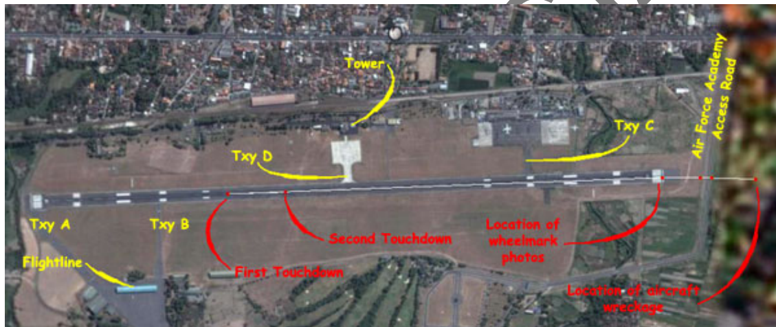
The path of PK-GZC during the landing roll and overrun (Google earth)
